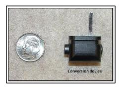
91. Either style of Glock switches works through the operation of a protrusion called a disconnector, which inserts into the slide from the rear: <sup>50</sup>
